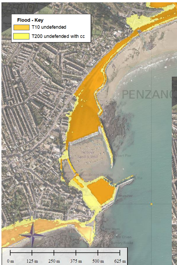
(a) Flood risk to Penzance Harbour area following failure of Harbour breakwaters
