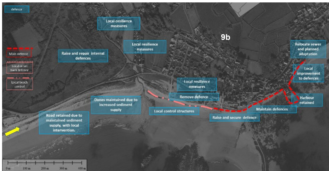
OPTION 9b Controlled realignment with the ability to adapt. (with additional sediment supply from west)
