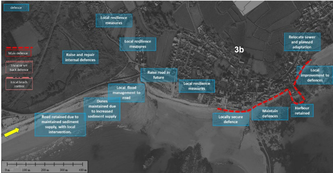
OPTION 3b Sustain core function of Town Adapt in other areas. (With additional sediment supply from the west)
