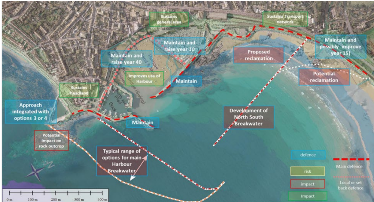
Figure 5-8. Schematic of Harbour Development approach (with implications for flood and erosion risk management).
